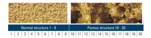
High-porosity grinding wheels provide the most favorable grinding procedure: self-sharpening, cold cutting, better chip removal, smaller force.
